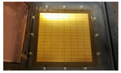
128 Pads of area 6x12 mm<sup>2</sup> have been used as anode
