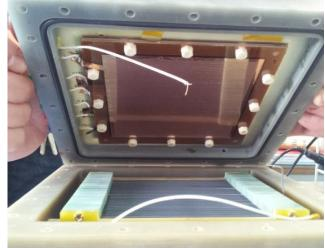
Assembly with Triple GEM detector
