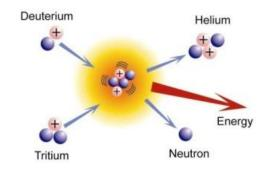
•They are not confined by magnetic field and can escape from the tokamak
