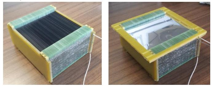
The full Lamella System. A total of 48 lamellas have been mounted mounted. Their distance is 2 mm
